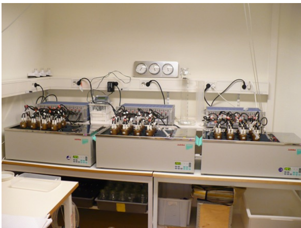
Image 5. Test tubes combining buffered ruminant fluid, feed and algae (0.5% on organic matter basis) at SLU labs.
