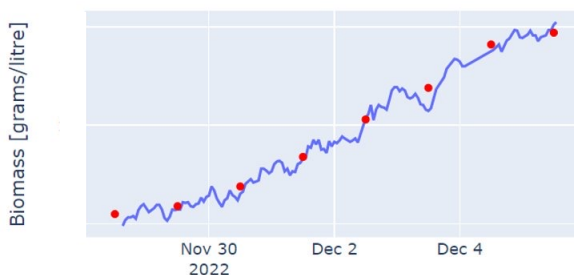
Figure 1. Continuous biomass readings (in blue) for one week of testing performed with the biomass sensor. Daily average shown in red.
